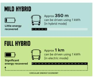
"Effectively, a full hybrid bus is a part-time electric bus, while a mild hybrid is just a more efficient diesel bus."
